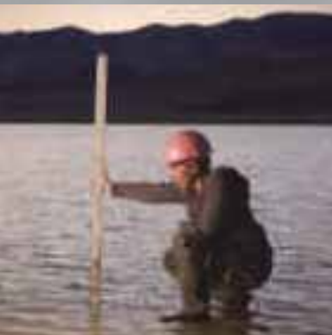
Rockwood's lithium business, Chemetall, operates the only US-based operating lithium resource at Silver Peak, NV. Here a technician measures the water levels of the lithium salt ponds. Rockwood is expanding its Silver Peak operation and adding high-purity lithium hydroxide capability at its Kings Mountain, NC, plant to be ready for the new generation of batteries in electric vehicles.
